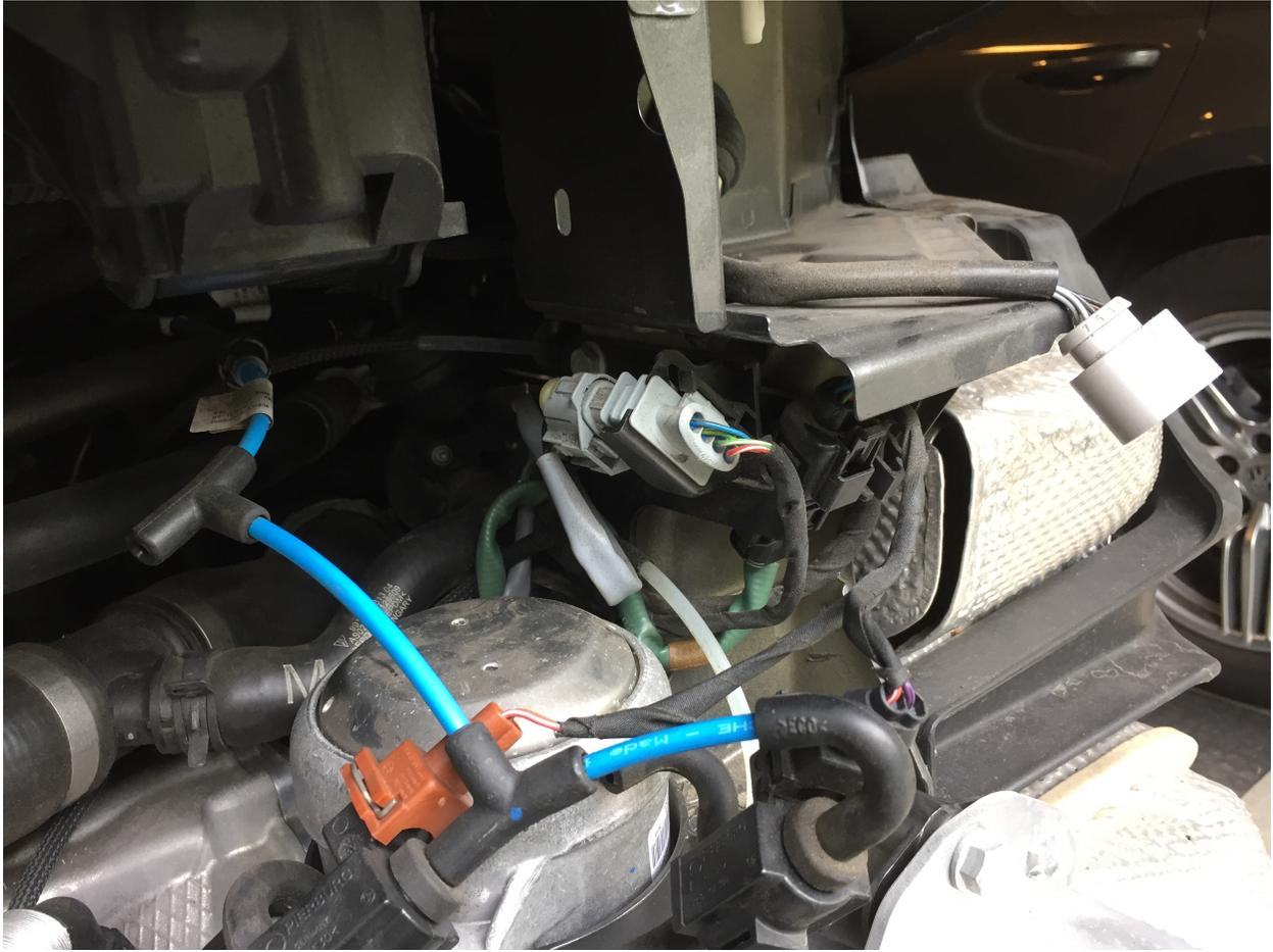
Repeat steps 5 and 6 for the other side. The driver side O2 sensor is more difficult because of a tighter fit with where the wire was routed.
