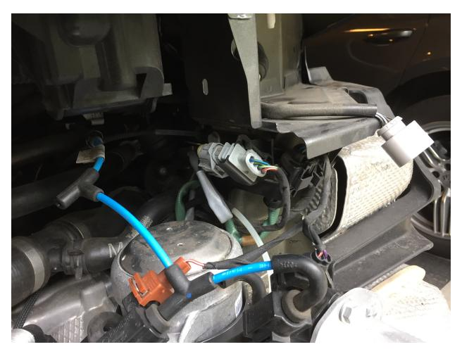
Repeat steps 5 and 6 for the other side. The driver side O2 sensor is more difficult because of a tighter fit with where the wire was routed.
