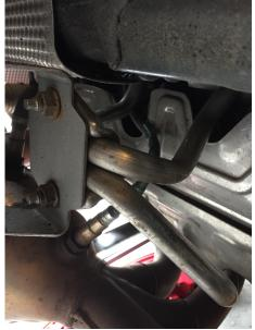
around and through where the old wire went, making sure to clip it into the holding clips as you go. Reconnect the new electrical connection. Replace wheel and lower jack. Torque wheel bolts to 118 ft lb.
