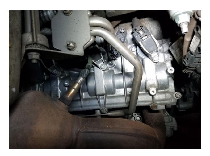
3. You'll see an electrical connector on each cylinder plugged into a coil-on-plug assembly. The connectors have a tab that has to be depressed (they click so you know you've released them). Push them off the coils. The COP on the left in this pic has been unplugged and removed with the electrical connector dangling, and the right one is still plugged in:
